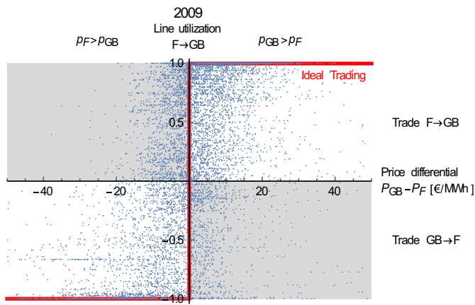
Fig. 1. GB France trading pattern – before market coupling: hourly capacity utilization of the France GB interconnector vs. hourly price differentials on the day ahead markets in 2009. Grey shaded areas indicate trading against the price differential.
